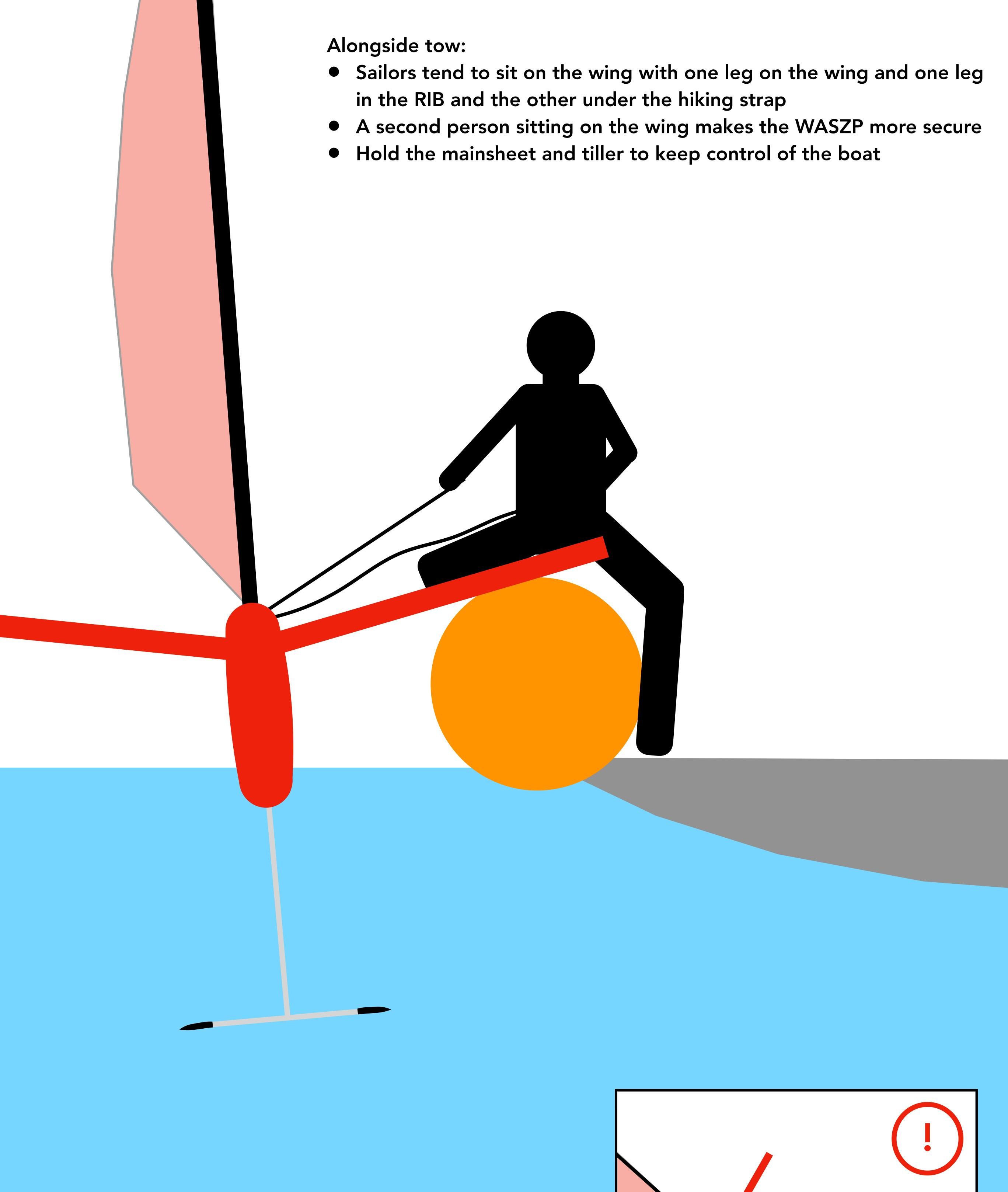
When you approach the WASZP, if the boat is heeled too much, the foils are close to the surface. The perfect heel has the leeward wing touching the water but not submerged. If the RIB tubes are wide, there is more risk of hitting the foils.
