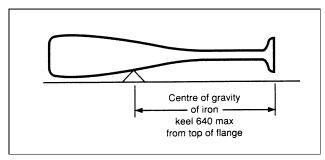
E.3.4.2 For boats first measured after 1st March 1994 the keel casting shall be weighed,
