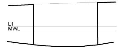
15.5.6 The two watertight bulkheads specified above may be replaced by a watertight cockpit. In this case the cockpit sole shall be above L1 level and the cockpit shall have at least two self-bailers. Openings for control lines shall meet the above requirements and any hatches shall maintain the watertight integrity of the cockpit. The weight of each bulkhead, including the weight of the adjacent ring frame if fitted, shall be not less than 6.5kg.
